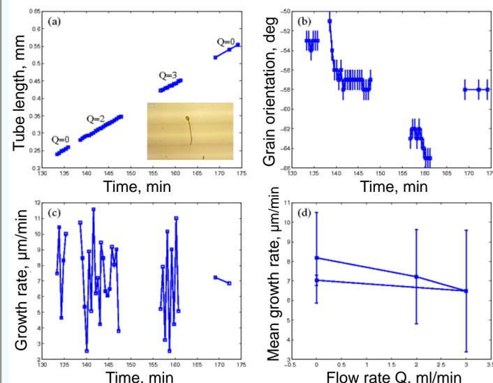
**Fig. 5.** Growth of a single pollen tube in the perfused microchannel; (d) indicates a reversible drop in the mean growth rate with an increase in flow rate  $Q$ .
