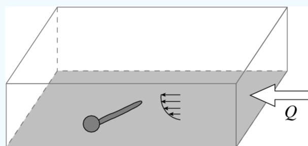
**Fig. 3.** Top: microchannel setup on the microscope stage; bottom: geometry of the channel (not to scale) with a pollen grain adhered to the base.
