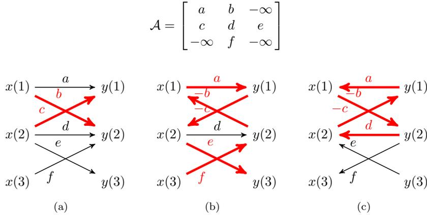
FIG. 1. (a) Bipartite graph  $G$  of  $\mathcal{A}$  with matching  $M = \{e_{12}, e_{21}\}$  highlighted with thicker lines. (b) Residual graph  $R_G(M)$  with directed path  $\sigma = \{e_{32}, e_{12}, e_{11}, e_{21}, e_{23}\}$  highlighted with thicker lines. (c) Transpose residual graph  $R_G^T(M)$  with cycle  $c = \{e_{12}, e_{22}, e_{21}, e_{11}\}$  highlighted with thicker lines.
