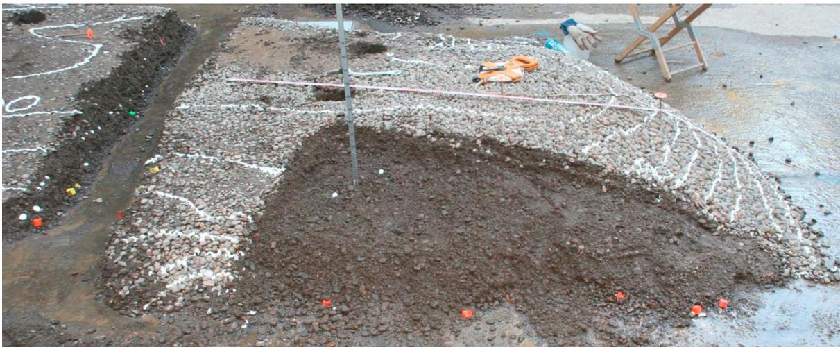
**Figure 17.** Photograph of the 27th August deposit termination. A layer of coarse-enriched surface material approximately 5 cm thick has been removed from a sector of the deposit, uncovering two white tracer stones. White lines on the undisturbed deposit surface are topographic contours, determined by laser leveling and applied with paste.
