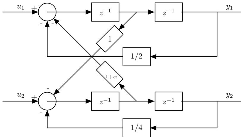
FIG. 4.7. Closed-loop system with feedback gains 1 and  $1 + \alpha$ .
